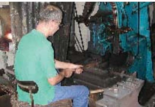
Mick Mylnek, a 38-year Henry Taylor employee, uses a hydraulic power hammer along with hand-forging to shape turning and carving tools.
