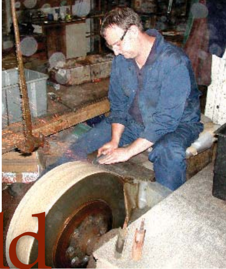
Andrew Triplitt, a 26-year employee at Crown Tools, straddles a large stone grinding wheel running in water to shape turning tools. His father also worked for Crown.
