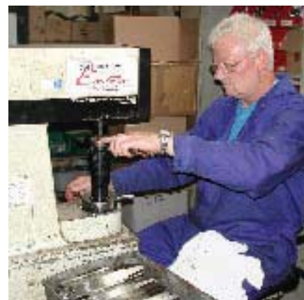
Mick Gibbs, a 20-year employee at Robert Sorby, tests each tool for hardness. Robert Sorby uses an industrial diamond to determine Rockwell hardness.
