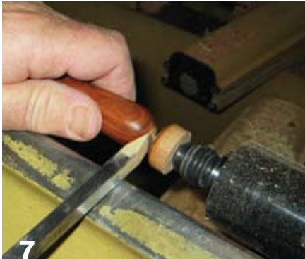
7 With a skew, separate the waste from the tailstock end.
