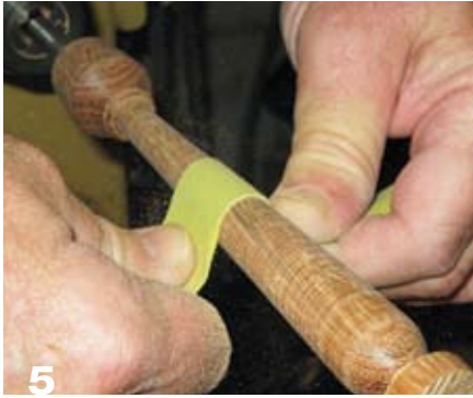
5 Sand the handle with 150 grit, then 180 grit and finish up with 220 grit.
