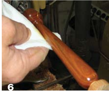
6 Apply a penetrating oil with paper towels. (Cloth rags present a safety hazard.)
