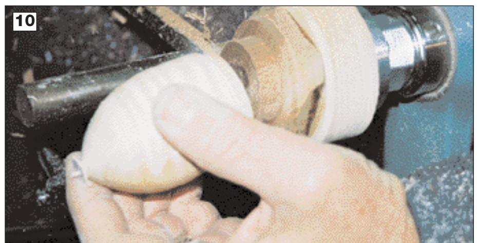
With a jam chuck turned from scrap material, mount the base, then turn the bottom of the acorn.
