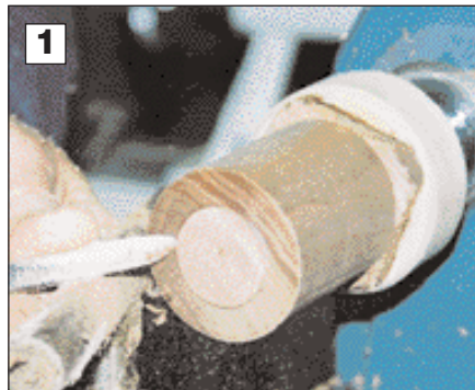
1 With a 3/8" spindle gouge, face off the end of the acorn lid.
