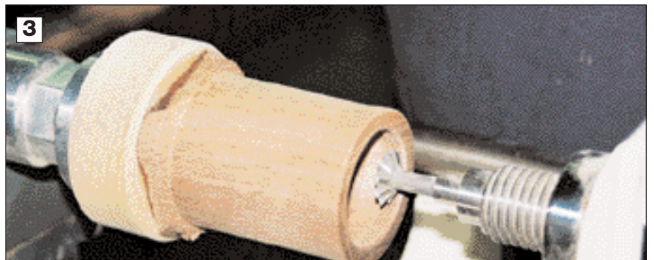
3 For the female threads, first check that the cutter just barely makes contact with the lid interior.
