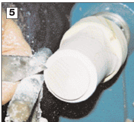
5 With a \frac{1}{16} " parting tool, turn the \frac{1}{16} " relief on back end of the tenon.
