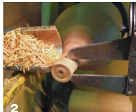
2 With a 3/4" spindle roughing gouge, turn the top of the ring holder to about 1/2" diameter.
