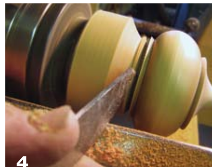
4 Define the bottom of the ring holder but don't yet part from the lathe.
