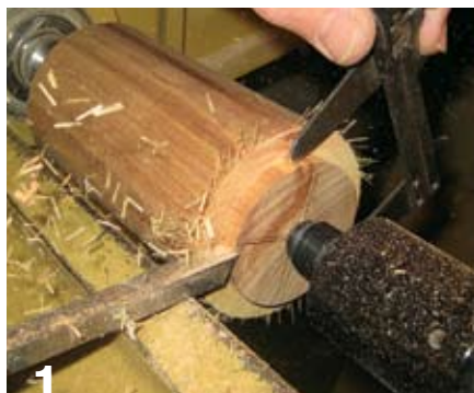
1 With a parting tool, create a 1/4"-wide tenon that is sized for your 4-jaw scroll chuck.
