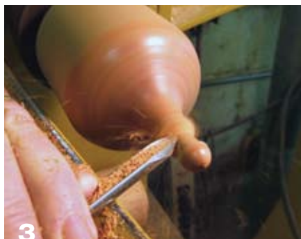
3 Use a spindle gouge to detail the top of the ring holder.
