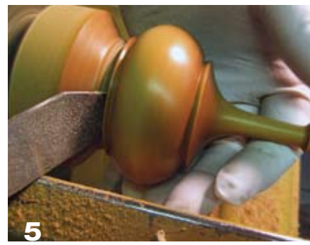
5 After the finish has dried, use a parting tool to undercut the bottom.
